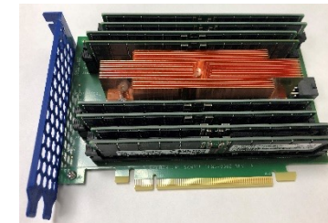
8-DIMM CXL AIC w/ 64GB DDR5 RDIMMs
