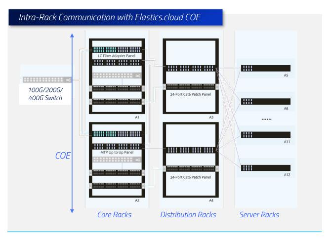
Ethernet wire eliminates cable bend radius limitations COE enables resource sharing/memory pooling within the rack
